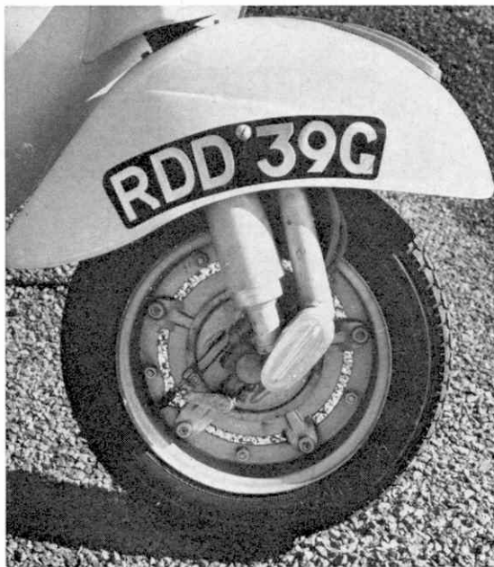
The large front mudguard prevents water from being thrown over the machine and rider in the wettest weather. Note the rather unusual suspension system.
