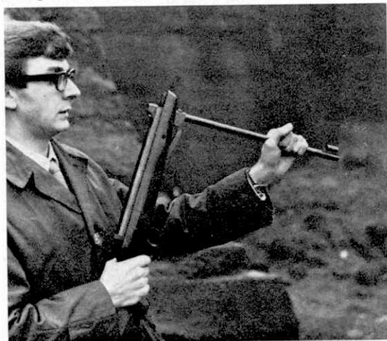
The majority of air rifles are cocked by breaking down the barrel as shown here. The pellet is loaded into the barrel at the same time.
