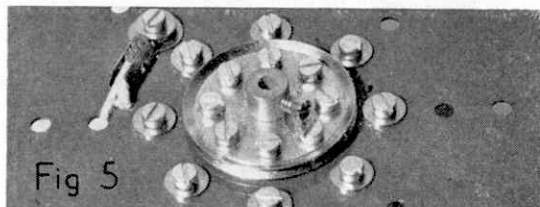
Fig. 5. A method of securing a heavy-duty winding cord to the outside of a winding drum. Note the use of a Rod and Strip Connector as a "thimble".
