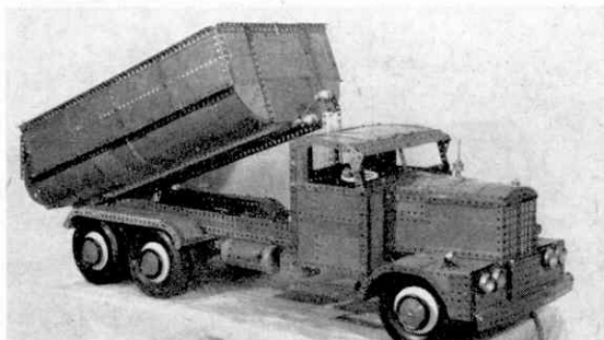
The many Meccano builders of Australia are represented here by Mr. B. R. Kuss of Nambour, Queensland, who designed and built this large, well-proportioned Tipper Truck fitted with many working features.
