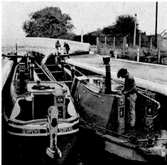
These two "narrow boats" are seventy feet long and only seven feet wide.
