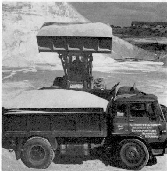
Ground rock salt being loaded into consumer's lorry at the Meadow Bank mine. Note the gigantic stock-pile in the background.
