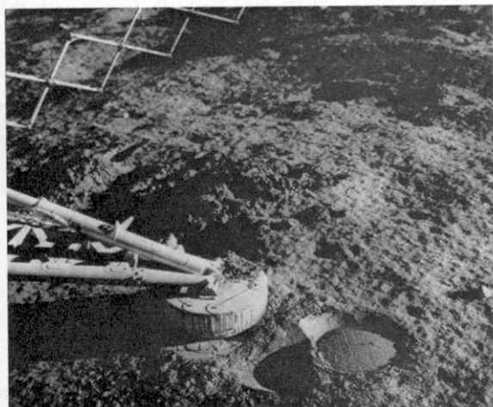
E: This close-up shot shows one of Surveyor 111's legs, and the 'bounce' imprint as it landed.
