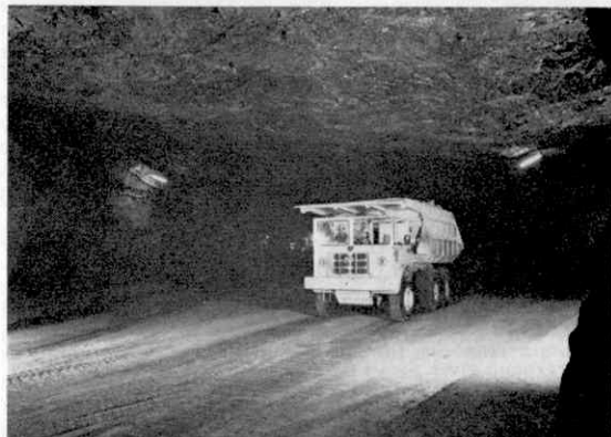
This 25-ton Foden diesel dumper is carrying salt from the rock face to the primary crushing plant.
