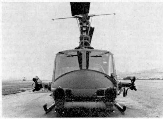
A United States Army Helicopter fitted with the new INFANT night-sight device.
