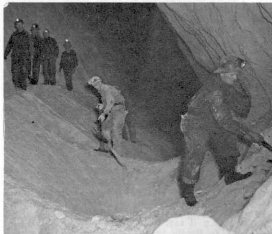
This picture was taken hundreds of feet down the Malagash salt mines, Nova Scotia, and shows miners shovelling salt into a tunnel where a scraper will collect it for dumping. Photograph: National Film Board.
