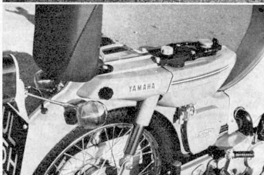
Top: The plastic legshields extend downwards to keep the worst of the weather off the rider's feet. Centre: The final-drive chain is totally enclosed. Lower: Access to the fuel and oil tanks is by lifting the dual-seat rearwards.
