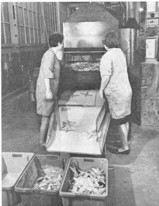
The "exit" end of the Phosphating Plant, through which Dinky Toy castings pass to be prepared for painting.
