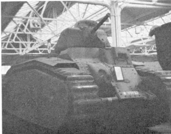
The M 2 Medium was a speedy machine which did not see action. Its chassis was used as a basis for the wartime M 3 Grant/Lee and M 4 Sherman.
