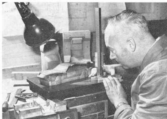
A Pattern-Maker at work, producing a large-scale wooden "mock-up" of the body component for a new Dinky.
