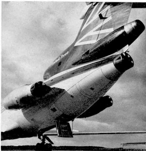
Close-up of the tail of a Trident Three in B.E.A. insignia, showing booster turbojet at base of rudder.
