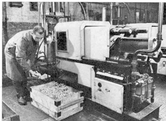
All Dinky Toy castings are produced on fully automatic, high-speed die-casting machines. Here, an operator is seen checking the output of one of the many machines at the Meccano Tri-ang factory in Liverpool.
