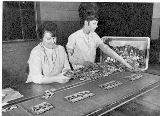
After all unwanted metal has been removed from the castings by "barrelling", the castings pass down an inspection conveyor. Any flash still remaining is removed by hand.
