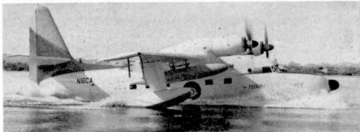
Conway Turbo Albatross re-equipped with Dart turboprop engines taken from a retired Viscount 700.
