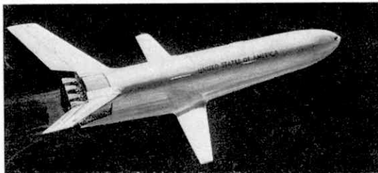
This aircraft, designed by General Dynamics, would be launched vertically. At the end of its mission it would re-enter the atmosphere and, using turbo-fan engines, cruise to an airfield to make a normal landing.
