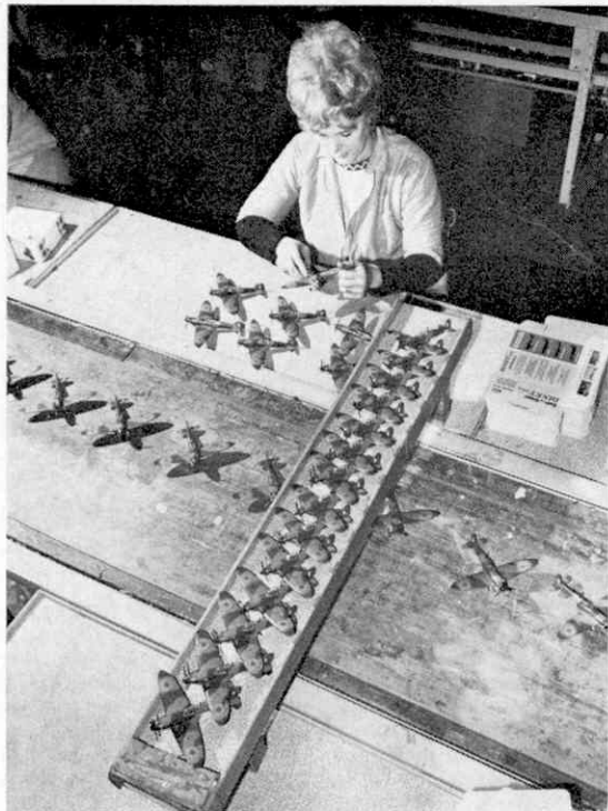
Finished Dinky Toy Spitfires being inspected and tested at the end of one of the Assembly Lines.
