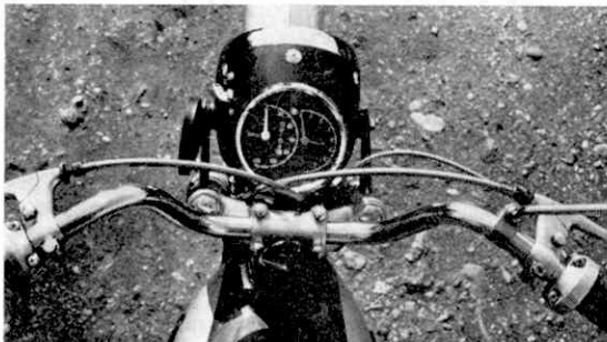
Neatly installed in one unit are the speedometer and rev. counter. The ignition switch can be seen on the left side of the headlamp.
