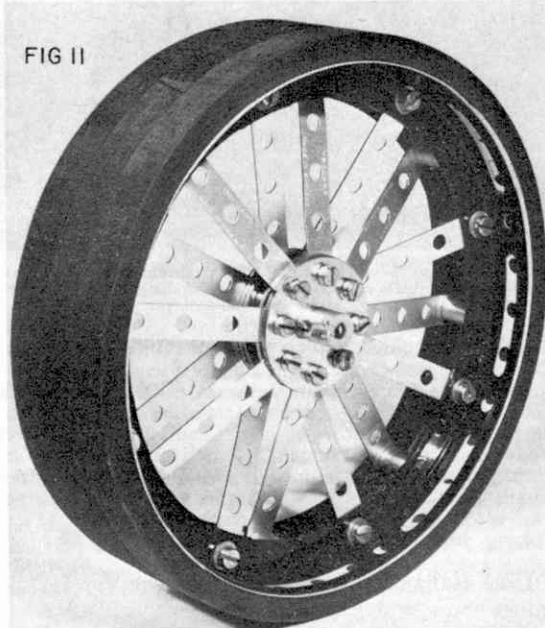
Fig. 11: A completed 16-spoke dished wheel for a Showman's Road Locomotive. The outer rim of the wheel is made from 5\frac{1}{2} \times 1\frac{1}{2} in. Flexible or Plastic Plates trapped by rubber tyres or bands.
