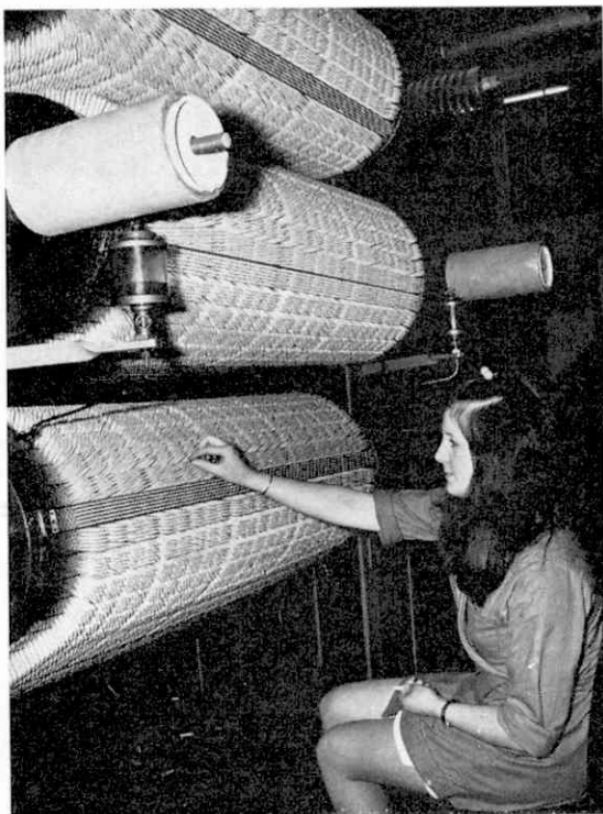
One of the four giant match machines. Here a girl is checking that all is well after the matches have been dipped in the composition that forms the head.
