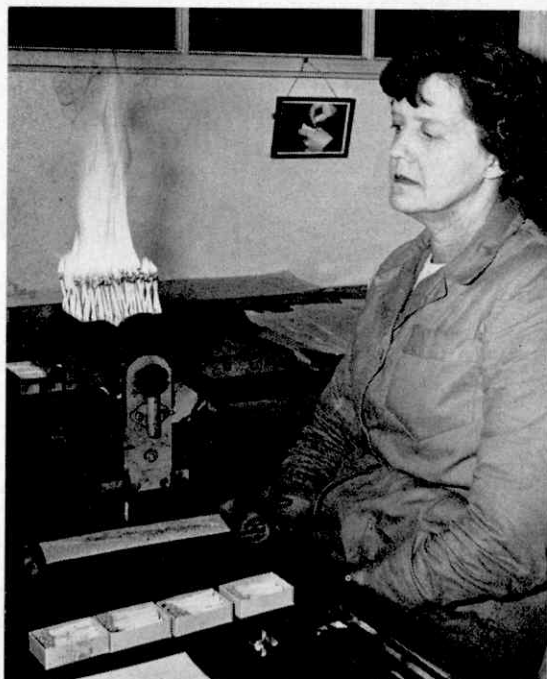
Testing finished matchboxes in accordance with British Standards.
