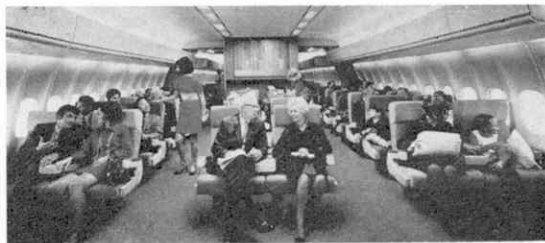
SPACIOUS DC-10 INTERIOR—Feeling of room-like spaciousness is created by expanded dimensions of McDonnell Douglas DC-10's wide-bodied fuselage. Cabin interior is 18 ft. 9 in. wide at passenger seat level and approximately 8 ft. high.
