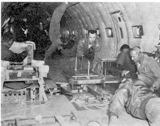
Airborne in more ways than one in the "Weightless Wonder", a KC-135 aircraft which flies parabolic patterns and helps train astronauts and develop tools for space use.
