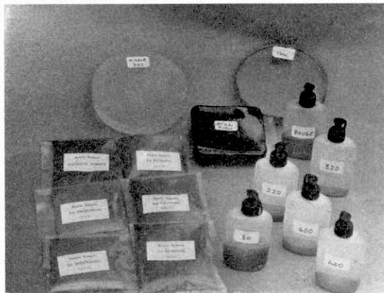
A typical do-it-yourself mirror making kit for a reflecting telescope. Photograph by courtesy of Austin Roberts Practical Optics, Birkenhead.
