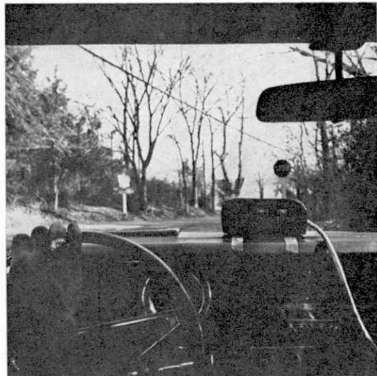
The electronic indicator on the dashboard projects signals to the driver in quickly-absorbed arrows and words.
