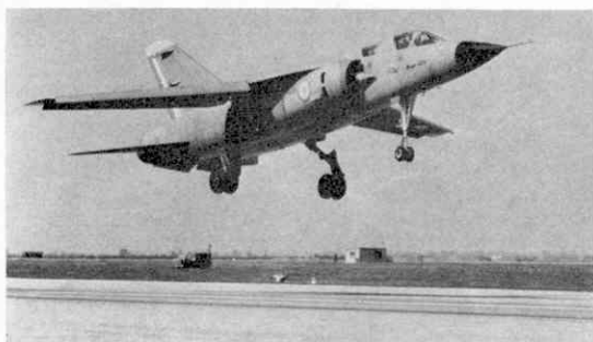
The Mirage G8 coming in to land; wings are fully forward and flaps and leading edge slats extended.
