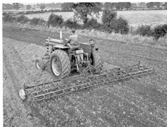
Top, a Ransomes TS89 four-furrow plough for use with four-wheel drive tractors. Centre, a 105 h.p. Massey-Ferguson 1100 tractor and the 24 ft. model MF37 spring tine cultivator. Bottom, Track-Marshall 70C crawler-tractor with Ransomes four-furrow plough, good on compacted ground.
