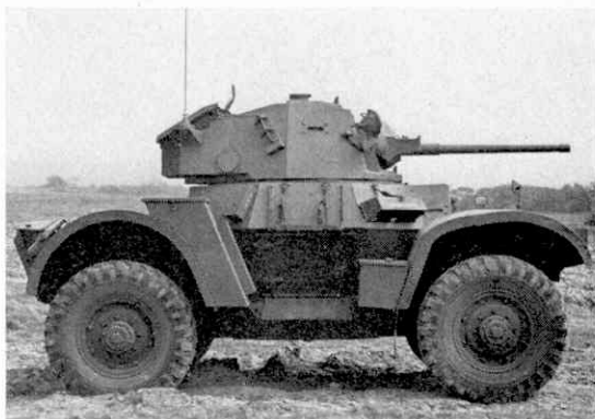
Left, the 7-ton Daimler 4 × 4 of WWII with fluid flywheel and five pre-selector gears forward or reverse! Speed 50 m.p.h., armament 2 pdr. cannon with co-axial machine gun. Dinky Toy No. 670 represents this vehicle.
