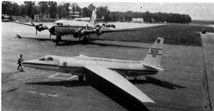
Left, one of the NASA U-2s being used to photograph test areas on the East coast of the U.S.A. using four 70 mm cameras.
