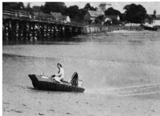
Distinguished group at the judging of the Pocket Meccano Competition (left) and, below, the Cyclone 274 light hovercraft, which will carry a load of 200 lbs.
