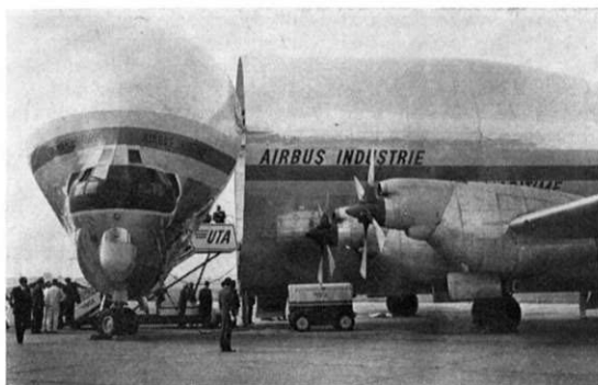
Above, Airbus Industrie, the management organisation for the construction of the A.300B European Airbus, has taken delivery of an Aero Spacelines Guppy-201. It will ferry parts of the Airbus to the final assembly line at Toulouse.
