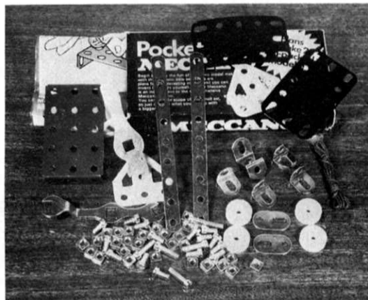
Fig. 3. Samples of both neat and ugly nut and bolt construction. Note neat alignment of boltheads in left-hand Flat Trunnion and the bad scoring of right-hand Flat Trunnion by poor Spanner work.
