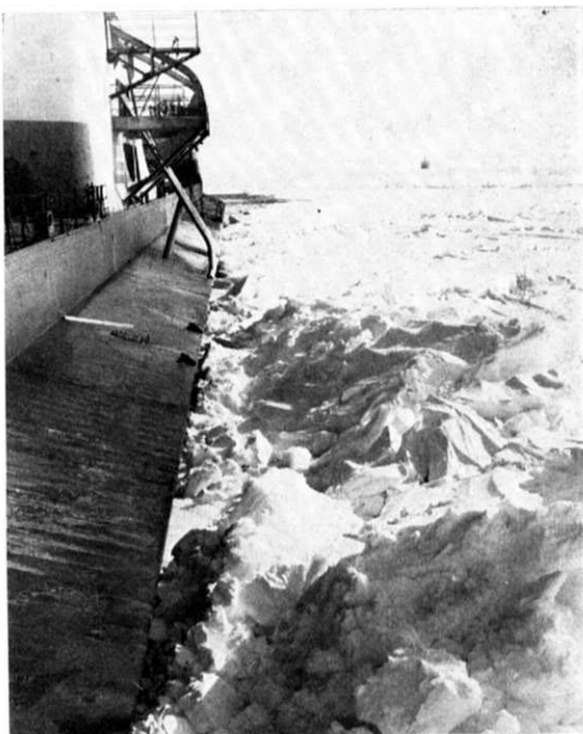
Right, The Manhattan trapped in heavy ridging ice in a northern area of Baffin Bay. Beyond is the new Canadian Coastguard icebreaker Louis S. St-Laurent which later moved in along the tanker to ease pressure and allow the ship to move again.
