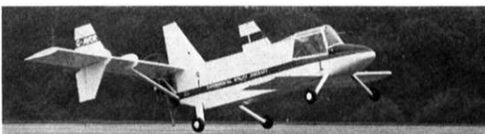
Above and below is the Lockspeiser LDA-01 utility prototype. The third fin, which can be seen in the photograph just above, was removed after initial flying trials. Small-scale flying models were used in the early stages of the design.
