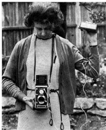
Left, showing how a flash, using an extension lead, can be held off the camera. Using the flash in this way leads to better modelling and does away with the "harsh" lighting of flash used direct on camera.
