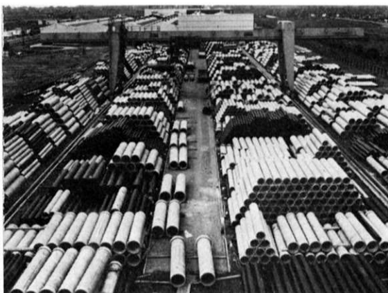
The stock area for asbestos-cement pressure pipes and pipes for sewerage and drainage in the Ditton (Lancs.) factory of TAC Construction Materials Ltd.
