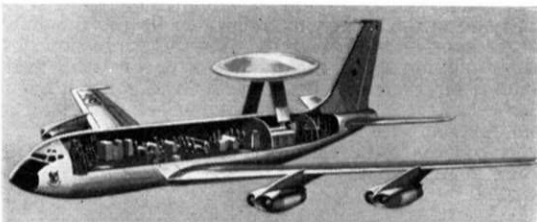
Top, first prototype EC-137D. Above, a cut-away showing the spacious interior. Auxiliary power unit, power distribution centre, and remote electronics are in lower forward cargo compartment (not shown). Below, first prototype on test with Boeing's Sabre (the only civilian-registered example) monitoring.
