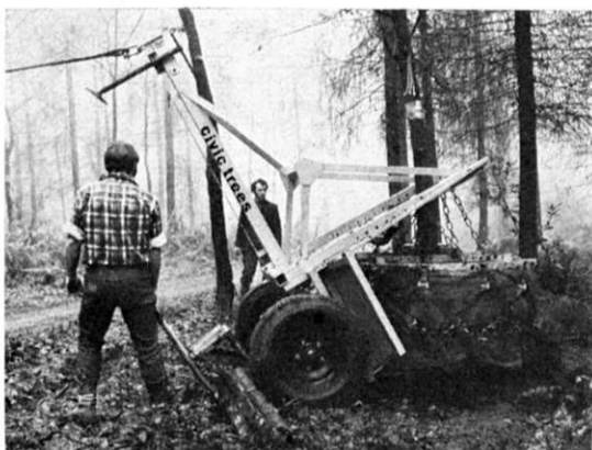
A Newman Civic tree mover loading a 2-ton beech at Epping, showing the tree rising and the root-ball wrapped in the special frame. Power is provided by the winch of the towing truck. Right shows the same tree loaded, with the head tied for transportation to its chosen site.
