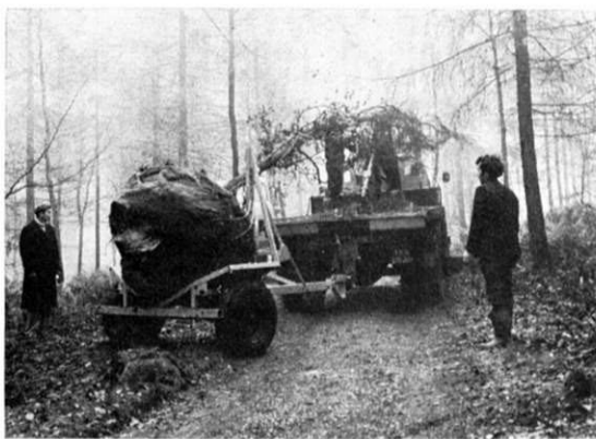
A Newman Civic tree mover loading a 2-ton beech at Epping, showing the tree rising and the root-ball wrapped in the special frame. Power is provided by the winch of the towing truck. Right shows the same tree loaded, with the head tied for transportation to its chosen site.
