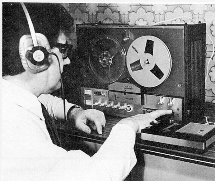
Fig. 2. The Author at work transferring recorded effects from cassette onto ¼" tape to form part of a permanent effects library. ¼" tape is much better to work with than a cassette as, in the latter, the tape itself is permanently enclosed and cannot therefore be marked for sound-track positioning.
