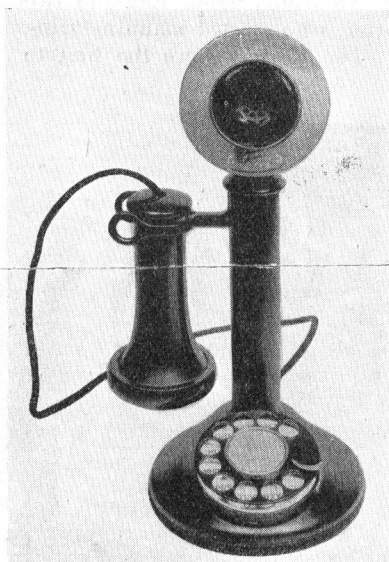
Fig 1 (left) A Standard Telephone Instrument equipped with the Dial for automatic operation.
