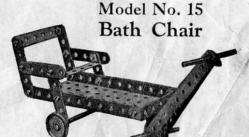
Parts | 1 of No. 16 | 13 of No. 37 required: 2 " " 17 | 1 " " 44 2 of No. 2 | 3 " " 22 | 1 " " 52 6 " " 5 | 4 " " 35 | 3 " " 60
