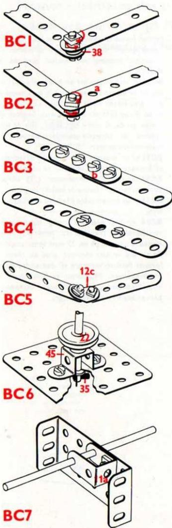
**BC1** is a method of joining two Strips together so that they can move in relation to each other. It is known as 'lock-nutting' and makes use of two nuts tightened together on the bolt. The nuts must not grip the Strips tightly.
