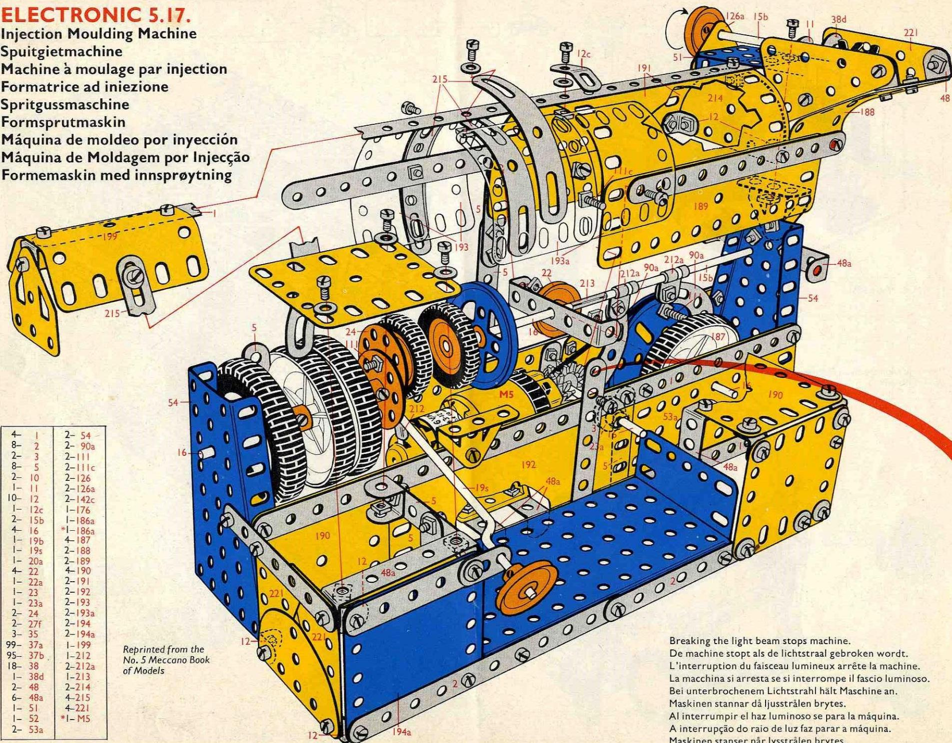
Breaking the light beam stops machine.
