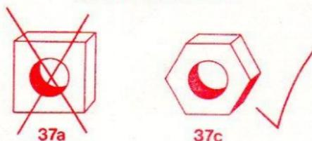
Please note that, since this Manual was printed, the square Nuts (No. 37a) illustrated in the model plans have been replaced by new, improved hexagonal Nuts (No. 37c). Where 37a is indicated, therefore, please substitute 37c.
