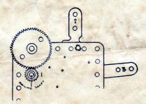
The motor will drive a large number of the smaller models without extra gearing. This diagram shows how extra gears may be added when more power is required. The wheel mounted on the driving-spindle is the ½" Meccano pinion; the wheel engaged by the pinion is the Meccano 56 toothed gear.
