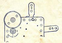
The motor will drive a large number of the smaller models without extra gearing. This diagram shows how extra gears may be added when more power is required. The wheel mounted on the driving-spindle is the  $\frac{1}{2}$ " Meccano pinion; the wheel engaged by the pinion is the Meccano 56 toothed gear.
