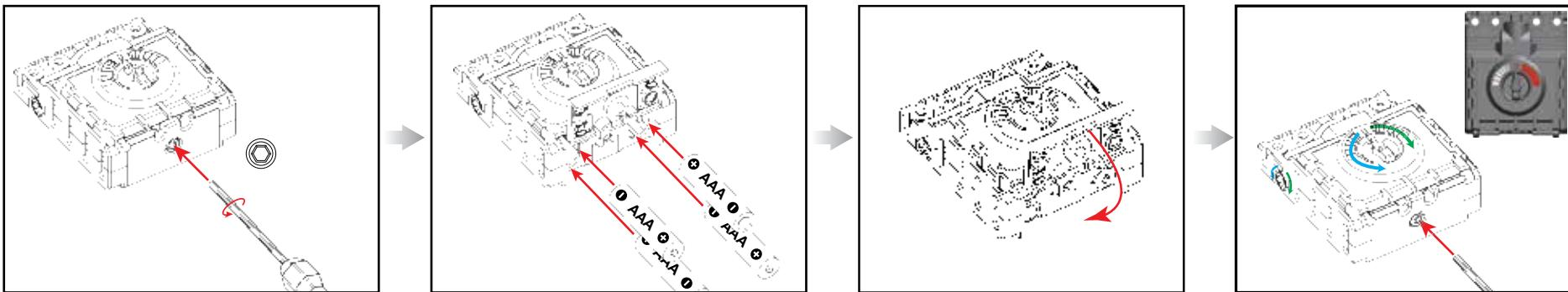
**EN HOW TO INSTALL BATTERIES:** 1. Open the battery door with a screwdriver. 2. If used batteries are present, remove these batteries from the unit by pulling up on one end of each battery. DO NOT remove or install batteries using sharp or metal tools. 3. Install new batteries as shown in the polarity diagram (+/-) inside the battery compartment. 4. Replace battery door securely. 5. Check your local laws and regulations for correct recycling and/or battery disposal.
