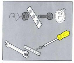
You have 4 different length screws. Most of the time use the No. 2 screw. Use No. 3 or No. 4 screws when you need a longer one. Use the No. 1 screw only with the disc or pulley to hold axles in place.
