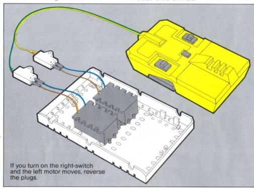
Look at the black plugs on the ends of the remote control wires. They are marked "+" (positive) and "-" (negative). Start by connecting the red wires from the motors to the "+" sides of the plugs and the blue wires to
