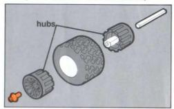
For the small tires (in sets 500 and 725), snap hubs together and slip rubber tires over them. Put in the axles, and add the hub caps.
