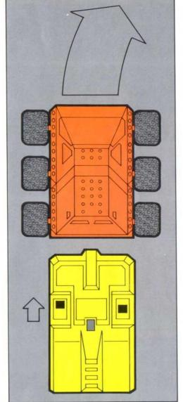
2) If the wheels still don't turn, pull the axles out of the motor and turn on again. If the motors work, check to see that you have the right axle support in place and that nothing is putting tension on the axle.
