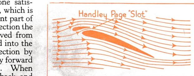
How the Handley Page automatic slot deals with the conditions shown in the upper right-hand drawing.
