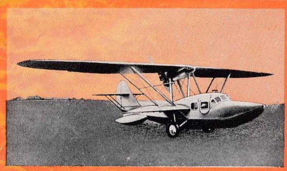
situated one in the bows and the other aft of the wings, and the pilot and navigator are accommodated in a small cabin in front of the wings. A Bristol "Pegasus VI" engine driving a pusher airscrew is mounted on a nacelle carried on struts between the wings.
