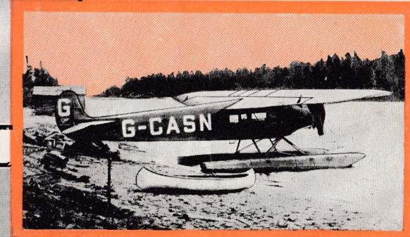
The Fairchild 82 single-engined high wing seaplane is a good example of this type of machine. It is extensively used on Canadian internal air routes and for air survey work. The twin-float undercarriage can easily be replaced by a twin-ski or two-wheeled one.
