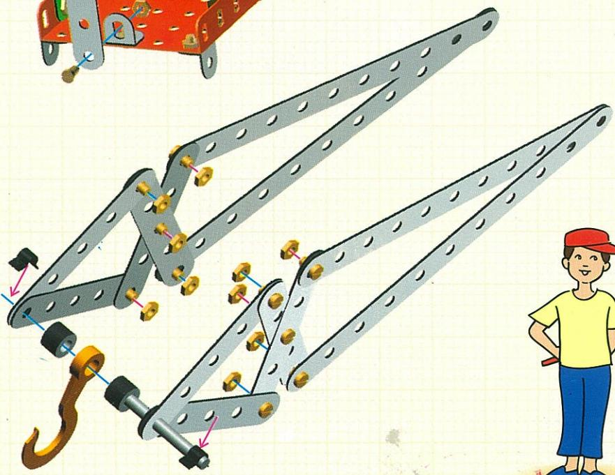
In this step, tighten all the bolts and nuts with hands. Do not over tighten them otherwise it will hinder the front back movement.
