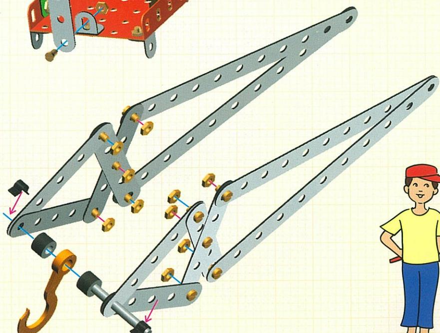
In this step, tighten all the bolts and nuts with hands. Do not over tighten them otherwise it will hinder the front back movement.
