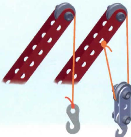
**USA** Simple and double arrangement of a string on a pulley wheel.
