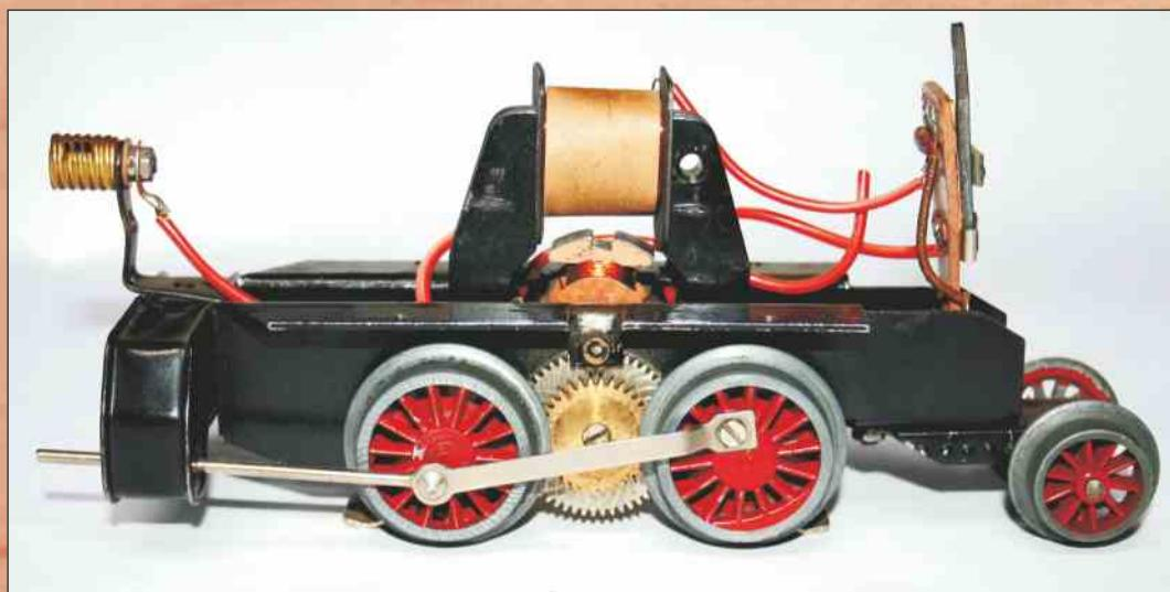
Construction of an old locomotive out of 1945. This AC motor, an own production and design, ensured very good driveability.
