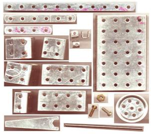
**The PARTS** These can be seen in a scan above, at 50% full-size. All holes are round. All corners not visible are square. Where not specified below the material thickness is between .050 & .055".
