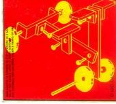
The parts are shown at the head of the next column. The blue ones are plastic with the Plugs originally attached to sprue (but much thinner than for the Wheels). The metal pieces are bright plated, probably nickeled, a few rather patchily. They are about 1mm thick, 7.5-7.7mm wide, & their corners have a small chamfer. Quality is adequate except that the bends are 5-10° short of 90°. The holes are at 7.5mm pitch and are mostly 3.4mm Ø, with a few
