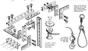
use in allowing other 'strip' parts to slide in them. The Spool, which is used as a winding drum, is probably wooden because the Ratchet has to be fastened to it with small tacks. No axles are mentioned and the wheels appear to run on long bolts locknutted to the chassis.
