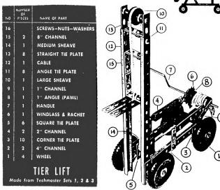
The main point of interest is the use of shallow channel girders, up to 16 holes long, as the main structural members, joined by 3 types of 4-hole brackets, and also their
