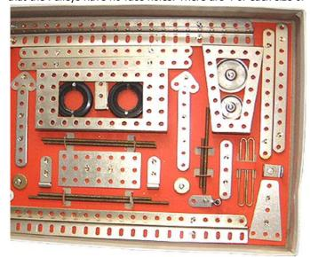
Flexible Plastic Plates on the small card. The parts are well made except that the gold paint is flaking off the 14 & 28t metal Gears. As might be expected from a STABIL inspired system the holes are 4.2mm  $\emptyset$  at 12.5mm pitch, and the thread is  $\frac{5}{32}$ " BSW. The hex Nuts though are a little larger than STABIL. No Trunnion of any sort was in the Set.
