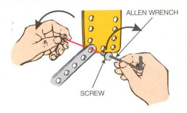
PLACE A SCREW ON THE END OF THE ALLEN WRENCH, AND PUT THE SCREW THRU THE HOLES AS SHOWN. THREAD NUT BY HAND ONTO SCREW AND TURN CLOCKWISE TO TIGHTEN.
